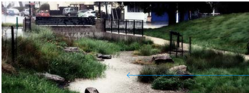
Rainwater capturing techniques: bioswale
